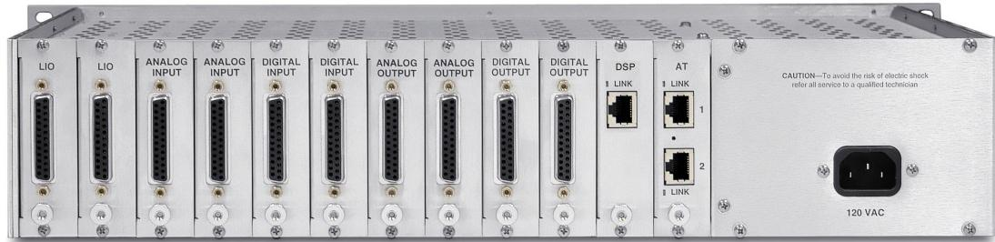
The E-SAT may be configured in a variety of I/O card complements using various combinations of analog and digital audio input and output daughter cards. All audio input, output, and logic connections are made via multipin DB-25 connectors located on the cage rear and mounted on the daughter cards. The daughter cards plug into the E-SAT's backplane connectors.
