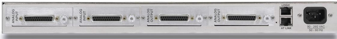
All audio input and output connections are made via DB-25 PCB-mounted connectors located on the rear of chassis. The factory supplied hand crimping tool is used for all DB-25 connections to and from the router (see instruction on page 1-16).
