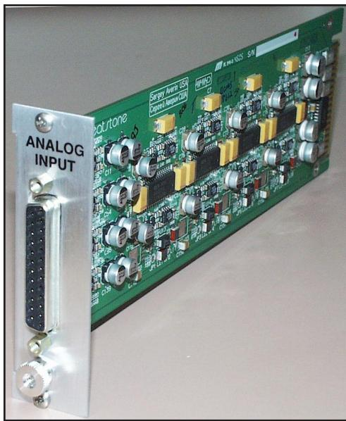
There are 12 ports on each logic card. Each logic card port may be configured as an input or output via an internal dipswitch selection. Analog and digital input and output cards each handle four stereo inputs/outputs. The E-SAT can support up to four input cards and four output cards, and digital and analog can be freely mixed. However, the card complement can not exceed 16 inputs or 16 outputs.
